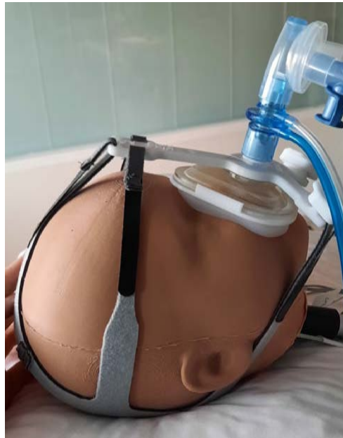
Testing personalized mask on test head models
